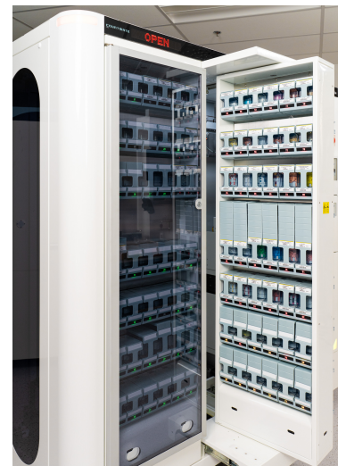
Pivoting sections allow for easy cleaning and maintenance.
