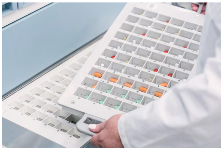
Special Tablet System (STS) tray for non-canister medications and partial pills.
