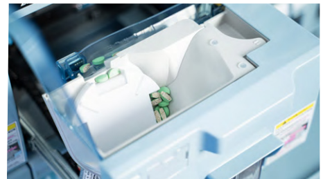
2 standard auto-canisters for partial tablet dispensing.
